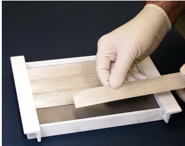
Figure 4. Hand Lay-up of MetPreg Tape
