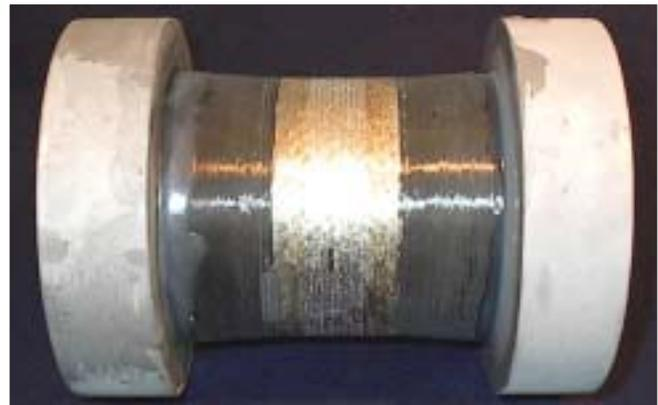
**Figure 4.** Test specimen for biaxial hydroburst testing.
