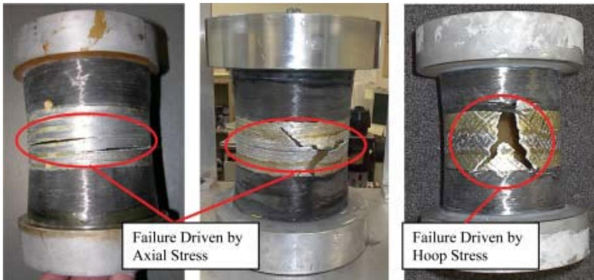
**Figure 7.** Biaxial hydroburst test failures: hoop-only (left), hoop-helical-hoop (middle), and helical-hoop-hoop-helical.
