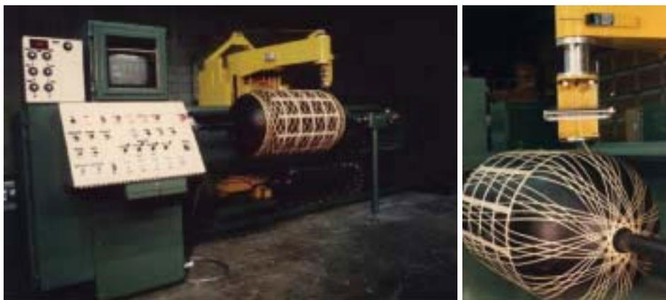
**Figure 1.** Composite filament winding.
