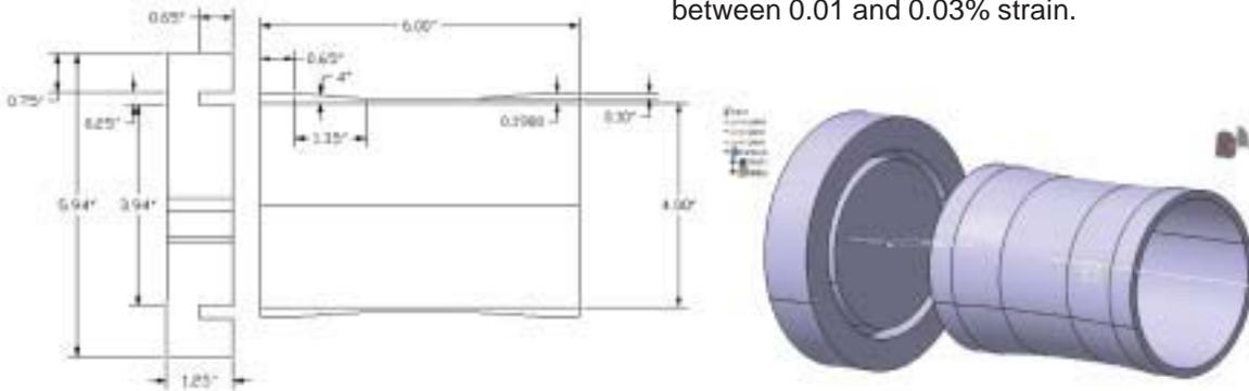
**Figure 3.** End closures for biaxial burst tests.
