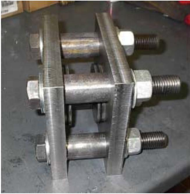
**Figure 2.** Uniaxial hydrostatic burst test fixture.
