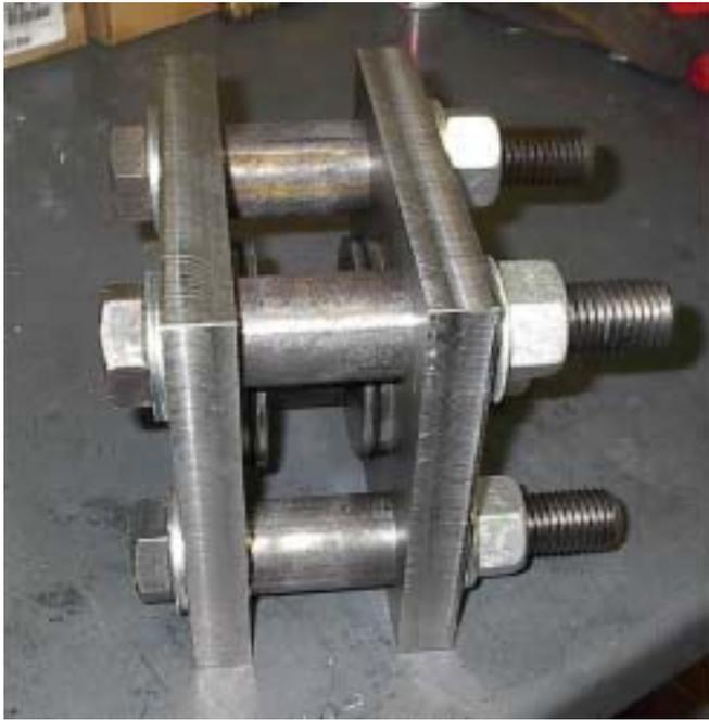
**Figure 2.** Uniaxial hydrostatic burst test fixture.
